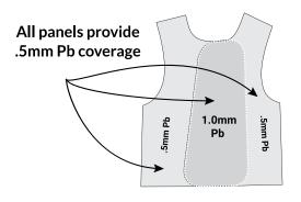
TYPE 2: Must be Overlapped to Protect
